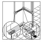
After completion of the door reversing operation, check that the door gasket adheres to the cabinet. If the ambient temperature is cold (i.e. in Winter), the gasket may not fit perfectly to the cabinet. In that case, wait for the natural fitting of the gasket or accelerate this process by heating up the part involved with a normal hairdryer on a low setting.
